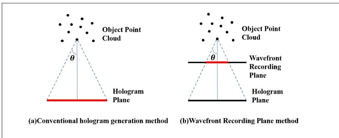
Fig 1. (a)conventional hologram generation method (b) Wavefront recording plane method
